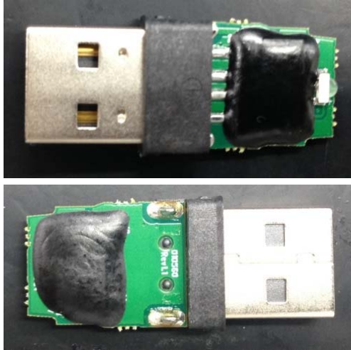
Figure 1 – eToken 5110 Crypto Boundary (Top and Bottom)
