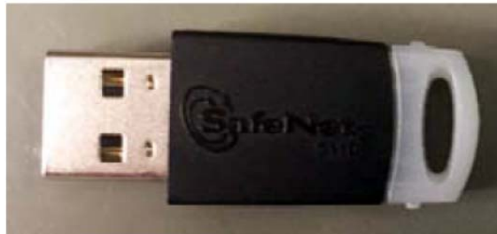
Figure 2 – Shows the Module with the outer enclosure, which is not within the cryptographic boundary
